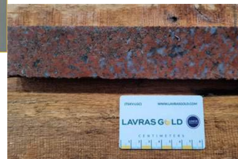
Perthitic Granite (alkali feldspar granite) forms when milky quartz precipitates in vugs. Chlorite, phengite, carbonate, sulphides, gold, REE replace milky quartz and forms episyenite
