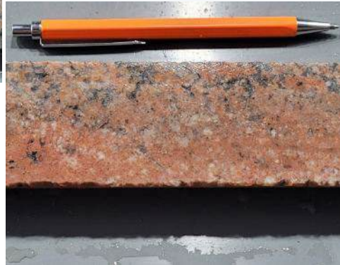
Unaltered granodiorite Original fresh granodiorite with microfracture showing incipient metasomatism
