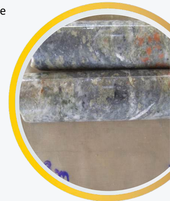
Gold typically occurs in pyrite, found in a matrix of silica and sericite.
