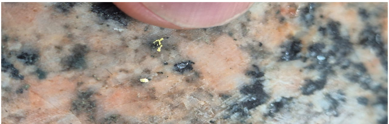
Figure 3 – Visible gold (bright yellow) in association with magnesium rich sphalerite (grey – metallic) in hole 25CN016
