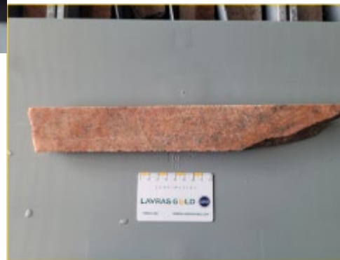
Albitite - Original granodiorite completely altered by metasomatic processes resulting in volume loss
